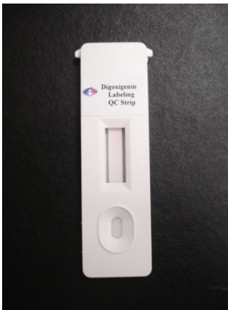
Figure 3- An example of a control strip with no color development, 0.5 \mu L of Unlabeled Mouse IgG was transferred onto the center area of the membrane of the QC Strip and then 100 \mu L of QC Buffer was transferred into the sample well of the QC Strip.
