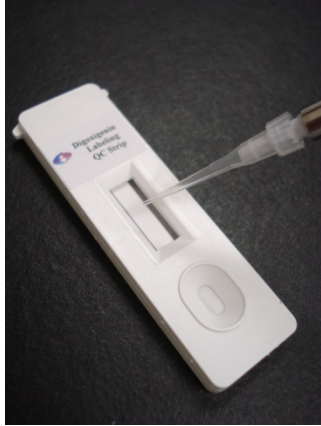
Figure 1- Transferring a drop of solution onto the center area of the membrane of the QC Strip
