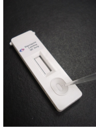
Figure 2- Transferring QC buffer to the sample well of the QC strip
